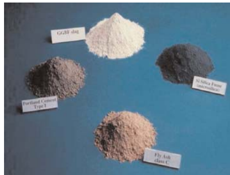
Figure 5: Comparison of various finely divided cementitious materials (Clockwise, from top: slag cement, silica fume, fly ash and portland cement).
